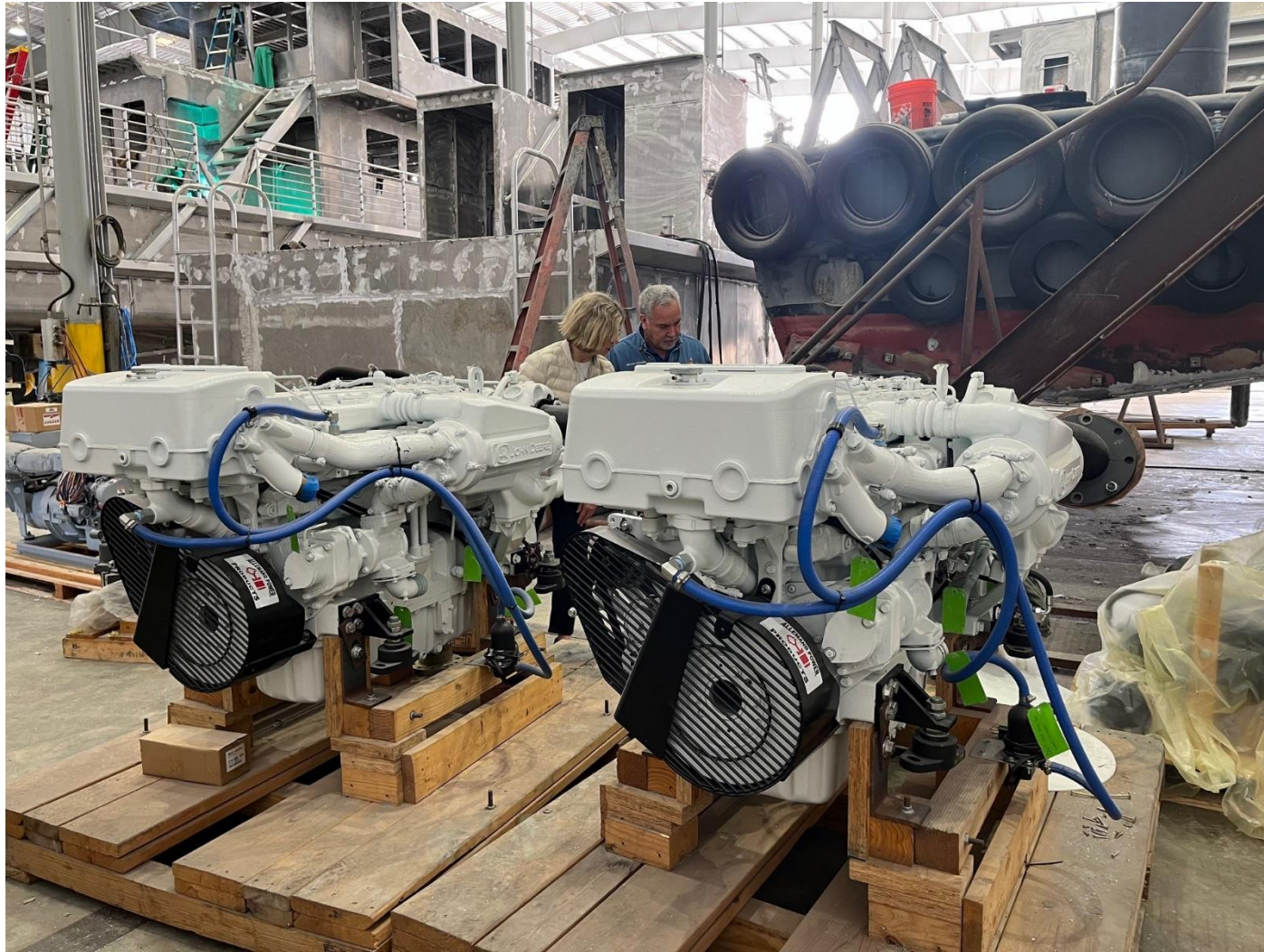
John Deere Marine Propulsion Engine - 6090SFM85 9.0L PowerTech™ 242-410 kW (325-550 hp) EPA Commercial Marine Tier 3
