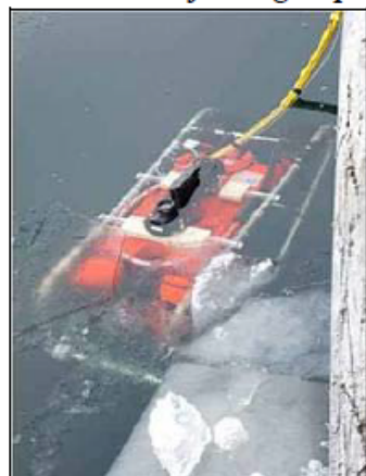
ROV in Process of Being Deployed
