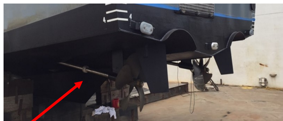
Spherical, sacrificial anodes were added to the Char's prop shafts to decrease galvanic corrosion on props and shafts.
